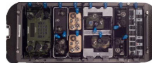
The capabilities of the modular and scalable Voyager deployable communications system extend beyond supporting traditional network modules to providing total RoIP integration for common soldier and backpack tactical radios. Custom made mounting brackets secure radios in place in the Voyager 8 transit case and chassis system.
